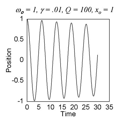
Amplitude drops by 1/e in  $Q/\pi$  cycles.
