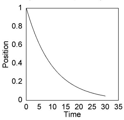
3 "Critically Damped": Q=0.5  $\gamma=2\omega_o$
